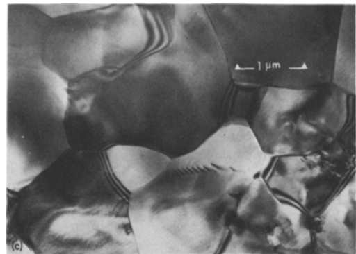
Figure 4 A comparison of triple-junction structure in (a) as-received, and (b) heat-treated ceramic B. The change in grain-boundary curvature and orientation in the heat-treated ceramic is visible in the low magnification image (c).
